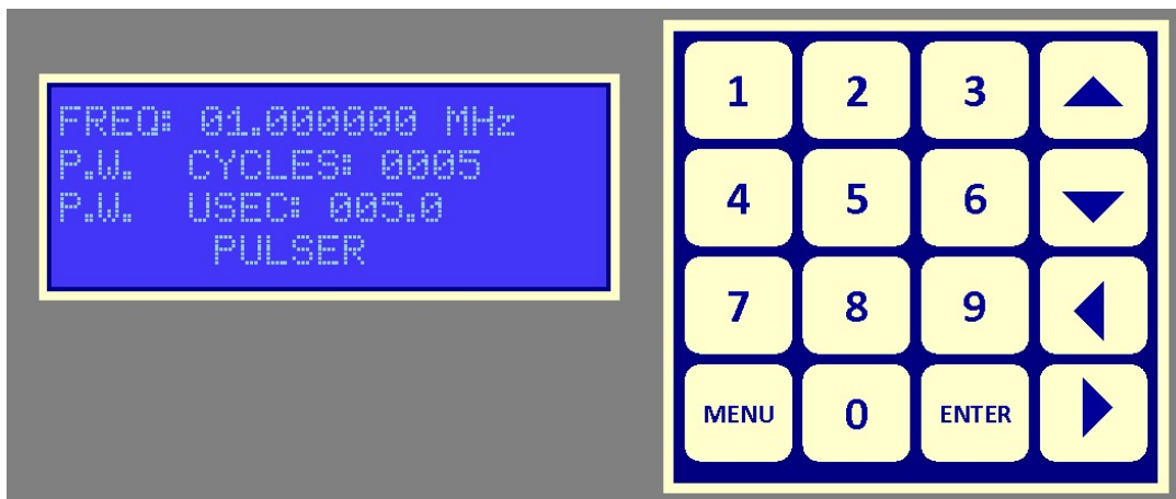
Figure 2.1: The keypad display console for manually controlling the RPR-4000.
