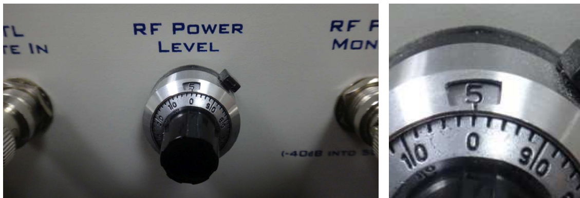
FIGURE 4: The main level, or gain, control for the GA-2500A is this 10 turn knob. When first getting started, set this to a mid-range value (5.00 is a good place to start)
